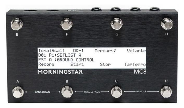
Welcome to your MC8 MIDI Controller. With this, you are able to control any device that accepts MIDI, regardless of brand or model. Each switch on your Morningstar controller can be programmed to perform any function you want.
