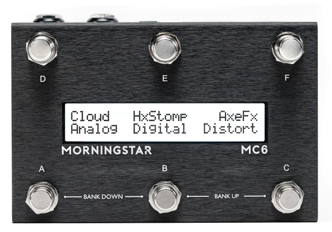
Welcome to your MC6 MIDI Controller. With this, you are able to control any device that accepts MIDI, regardless of brand or model. Each switch on your Morningstar controller can be programmed to perform any function you want.
